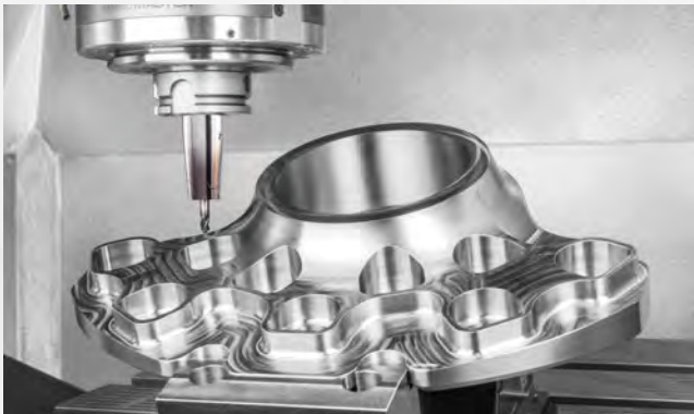
2: 20,000 rpm SK 40 motor spindle with 130 Nm | 35 kW (40 % DC)
