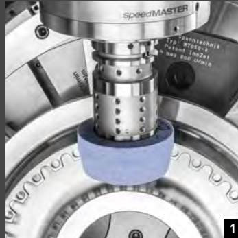
1: Spindle utilization for moving to component 2: Dressing with upright dressing tool
