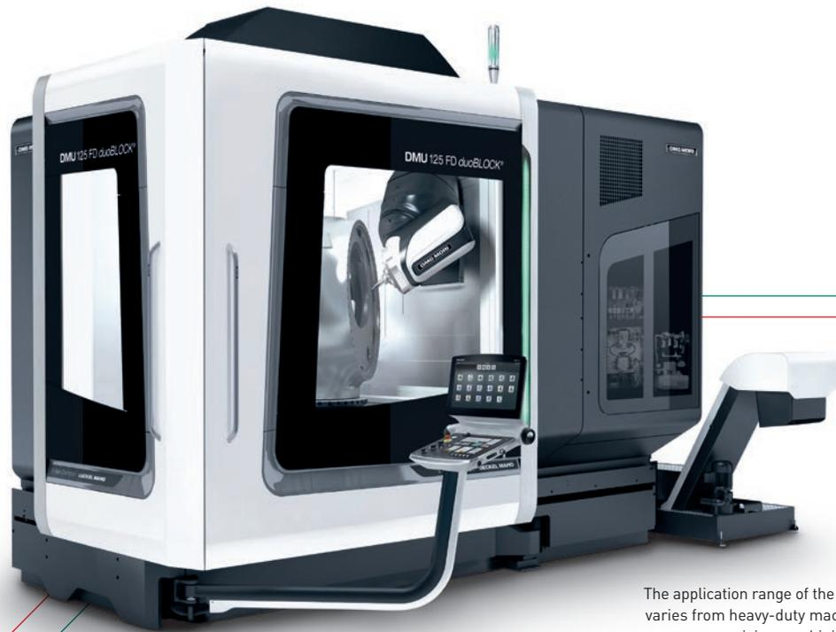
The application range of the DMU 125 FD duoBLOCK varies from heavy-duty machining through to µ-accuracy precision machining of seals for powertrains up to 1,600 mm in diameter in a wide range of materials from grey cast iron to chromium steel and bronze.
