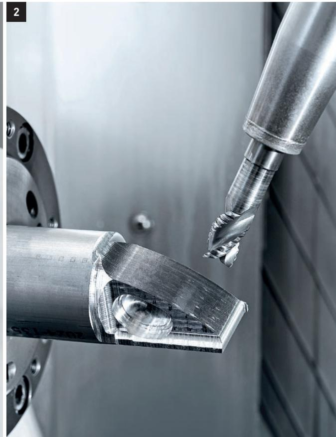
1.–3. The stability and cutting performance of DMG MORI machines enable high-precision machining of the complex prosthesis components from aluminium, steel or titanium.
