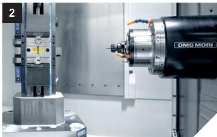
1. 6-sided complete machining on two NTX 2000 turn & mill machines from DMG MORI.
