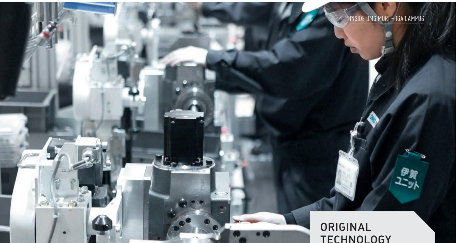
The Iga factory is characterised by a high level of vertical integration. This includes spindle production for the following series: speedMASTER, powerMASTER, torqueMASTER, compactMASTER and the turning spindle turnMASTER. Iga produces around 7,000 high-tech spindles a year.
